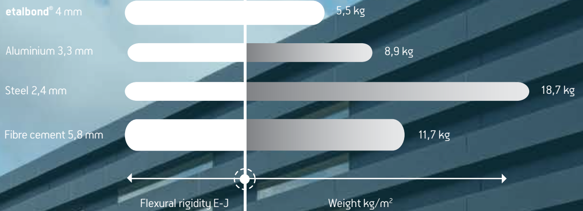
Comparison of thickness and weight with the same flexural rigidity
